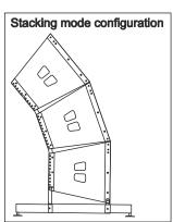
QREX can be installed stand-alone or in multiple configuration. Multiple installation of QREX can be done both in stack or fly configuration. Each loudspeaker has a fixing system that allows to be connected and secured to the other loudspeaker.
